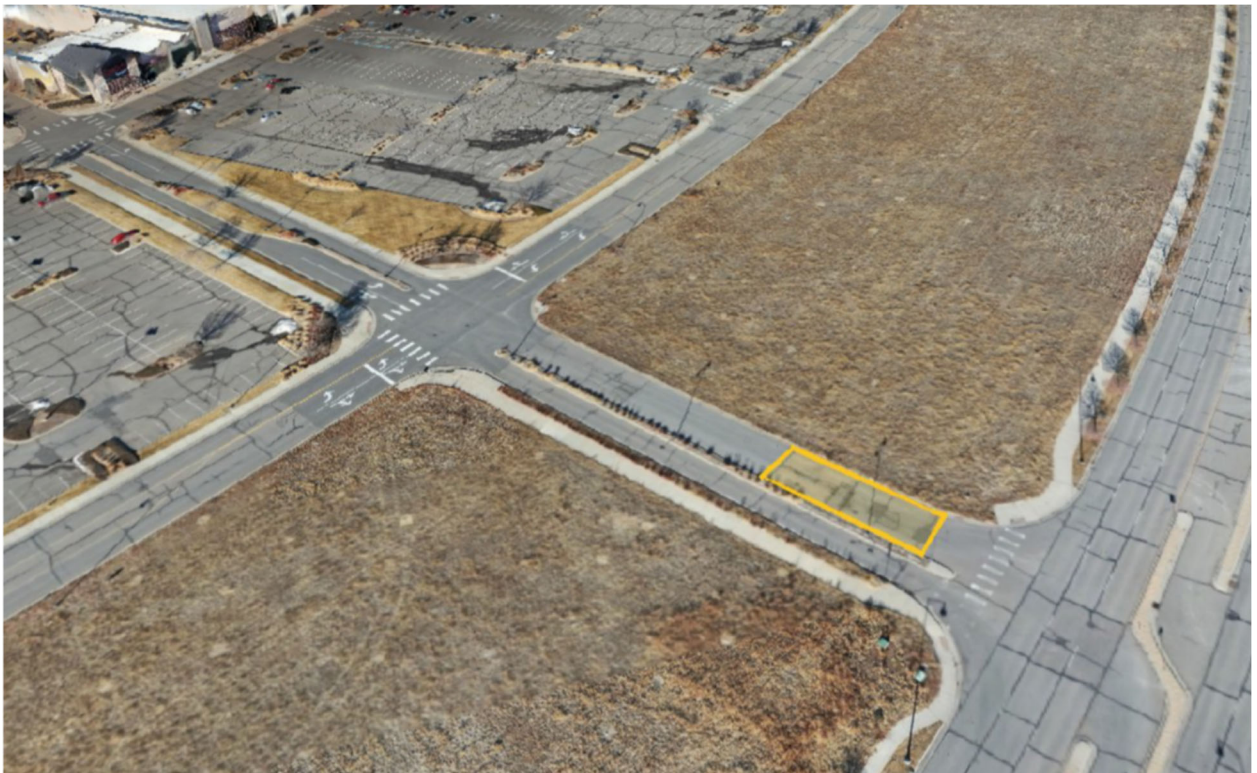
DARK ORANGE AREA - Asphalt Milling & Paving - 2"
