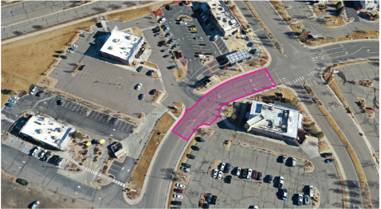
DARK ORANGE AREA - Asphalt Milling & Paving - 2"
