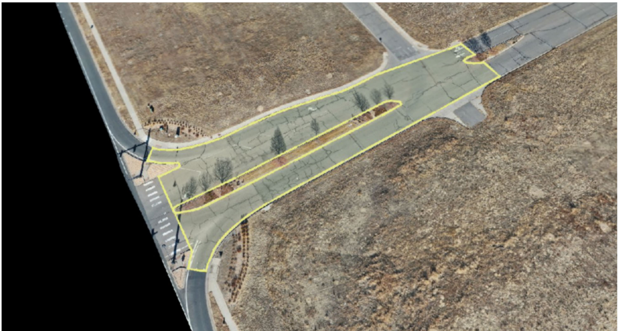
GREEN AREA - Asphalt Milling & Paving - 2"
